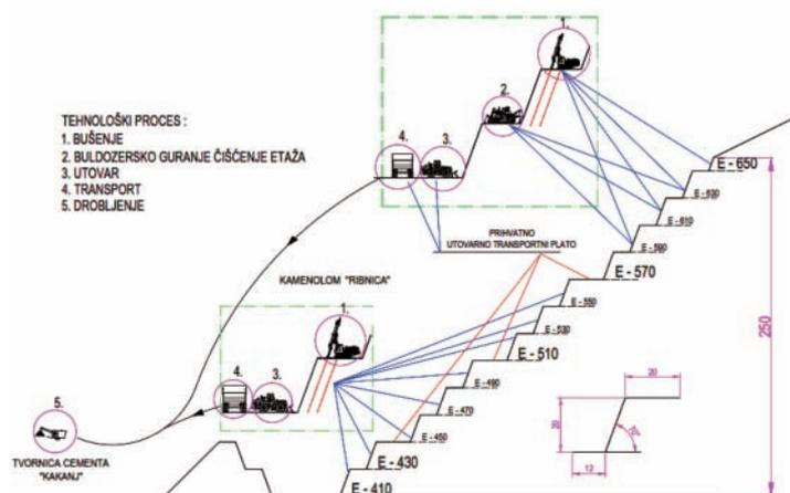
**Figure 2.** The primary technological scheme for obtaining limestones at the “Ribnica” quarry
