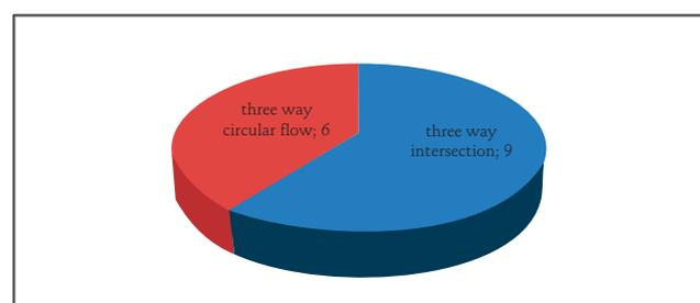
Figure 6. Conflict points of the three-way intersection and triangular circular flow
