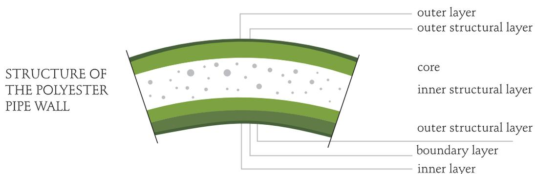
Figure 1. Structure of the polyester pipe wall
