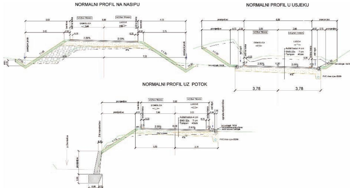
Figure 10. The characteristic cross-section of the analyzed variants of the connecting road for R473 and R474
