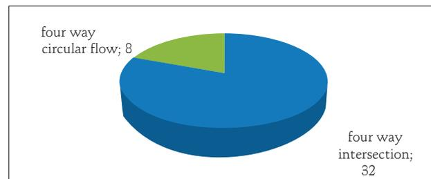
Figure 5. Conflict points of the four-way intersection and four-way circular flow
