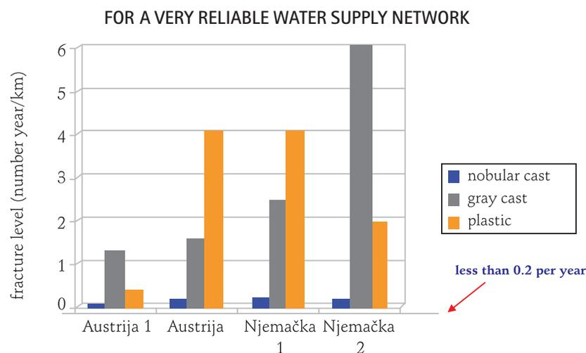
**Figure 2.** Fracture level of pipes of various materials in the water supply network
