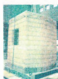
Real 3d model tested on the ISMES shaking table
