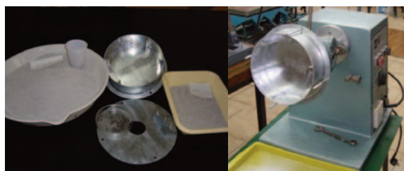
Figure 3. Drum for testing the wear resistance of pellets
