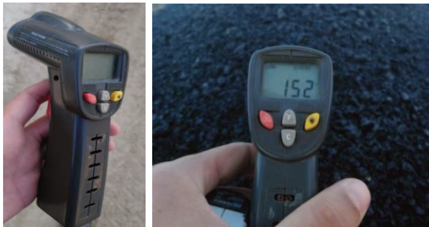
Figure 1. Second remote thermometer for measuring asphalt temperature at the place of production and at the place of installation
