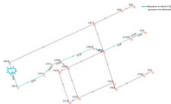
Figure 7. Simulation of methane outburst at the longwall [6]
