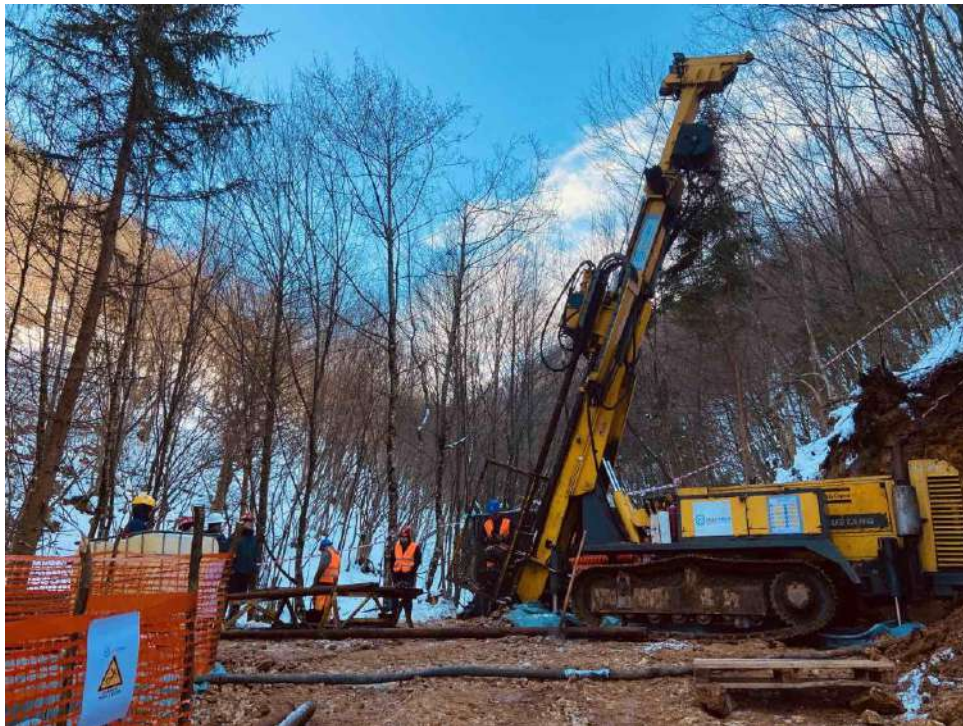
Image 2. Mustang 13 Atlas Copco Drilling Rig (Rig Teh East Sarajevo)
