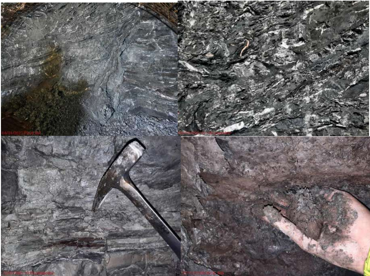
Figure 3. Structural properties (folding) of J/K flysch of the “Vrandučke serije” in the Zenica tunnel
