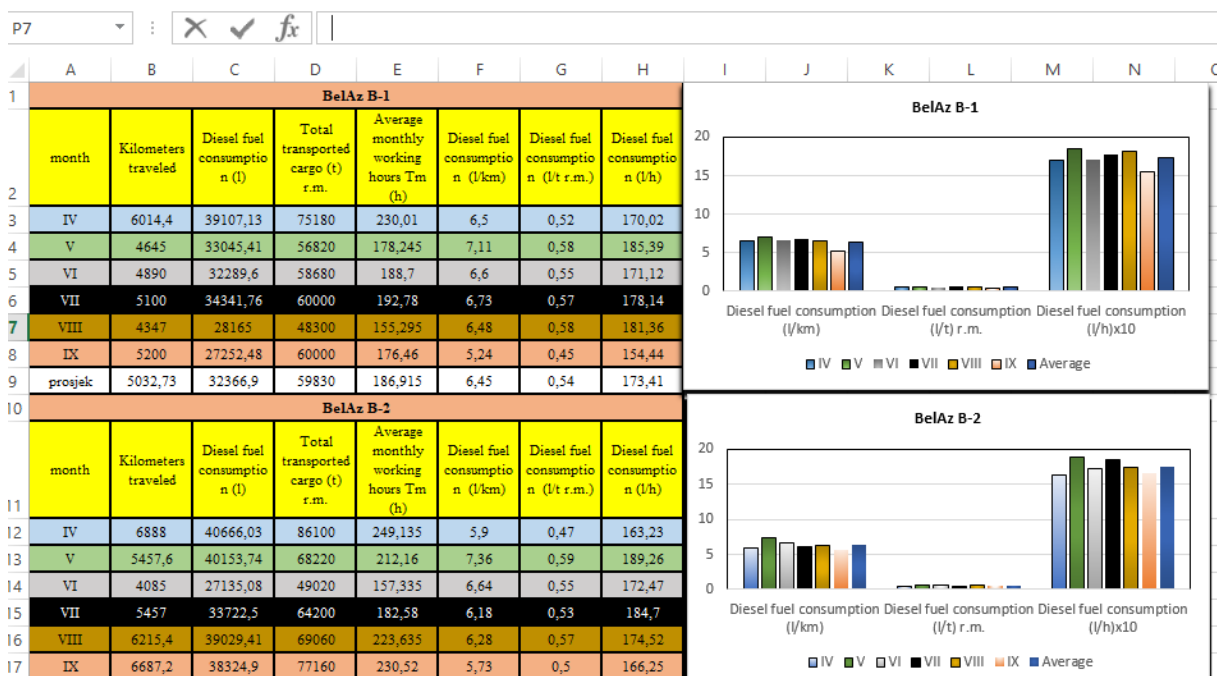
Figure 8 Consumption of diesel fuel (l/h), (l/ km), (l/t r.m.) in the IV, V, VI, VII, VIII and IX months
